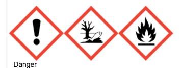
H319-Causes serious eye irritation. H336-May cause drowsiness or dizziness. H411-Toxic to aquatic life with long lasting effects. H222-Extremely flammable aerosol. H229-Pressurised container: May burst if heated.
