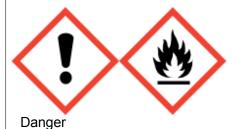
H319-Causes serious eye irritation. H336-May cause drowsiness or dizziness. H222-Extremely flammable aerosol. H229-Pressurised container: May burst if heated.
